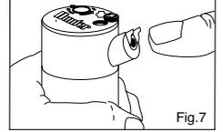
2. Using the hex key of the Hunter wrench, turn the radius adjustment screw (Fig. 6) counterclockwise to be sure it is not blocking the nozzle socket opening. If a nozzle is already installed, it can be removed by backing out the adjustment screw and turning on the water, or by pulling outward on the nozzle "ears" with a pair of needle-nosed pliers.
