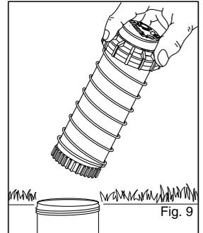
Another way to reset the right arc is to unscrew the body cap counterclockwise and remove the internal assembly from the body. Once removed, rotate the nozzle turret to the right stop, screw the internal assembly back into the body with the nozzle aligned to the right side of the area you want irrigated (Fig. 9). At this point you have realigned the right arc stop, and you can adjust the left arc to an appropriate setting.
